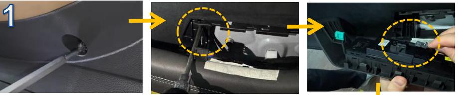
1. Door trim assembly process showing the connection of the window switch connector.
