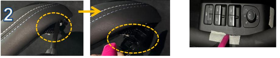
2. Door handle assembly process showing the installation of the lower blanking cover.
